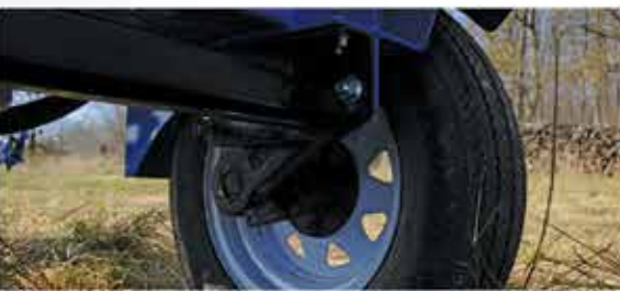
TORFLEX® Rubber Torsion Suspension Axles and 5.30 x 12 Highway Tires
